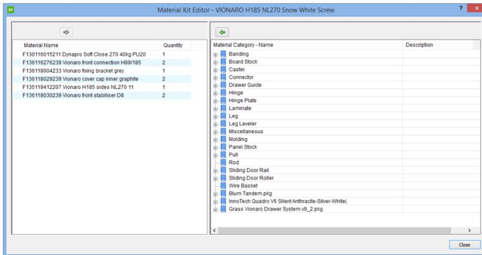
**NOTE: D8** is the default Stabilizer. If **D10** is required, replace the material from the Components folder. You will also need to change the boring dia.:
